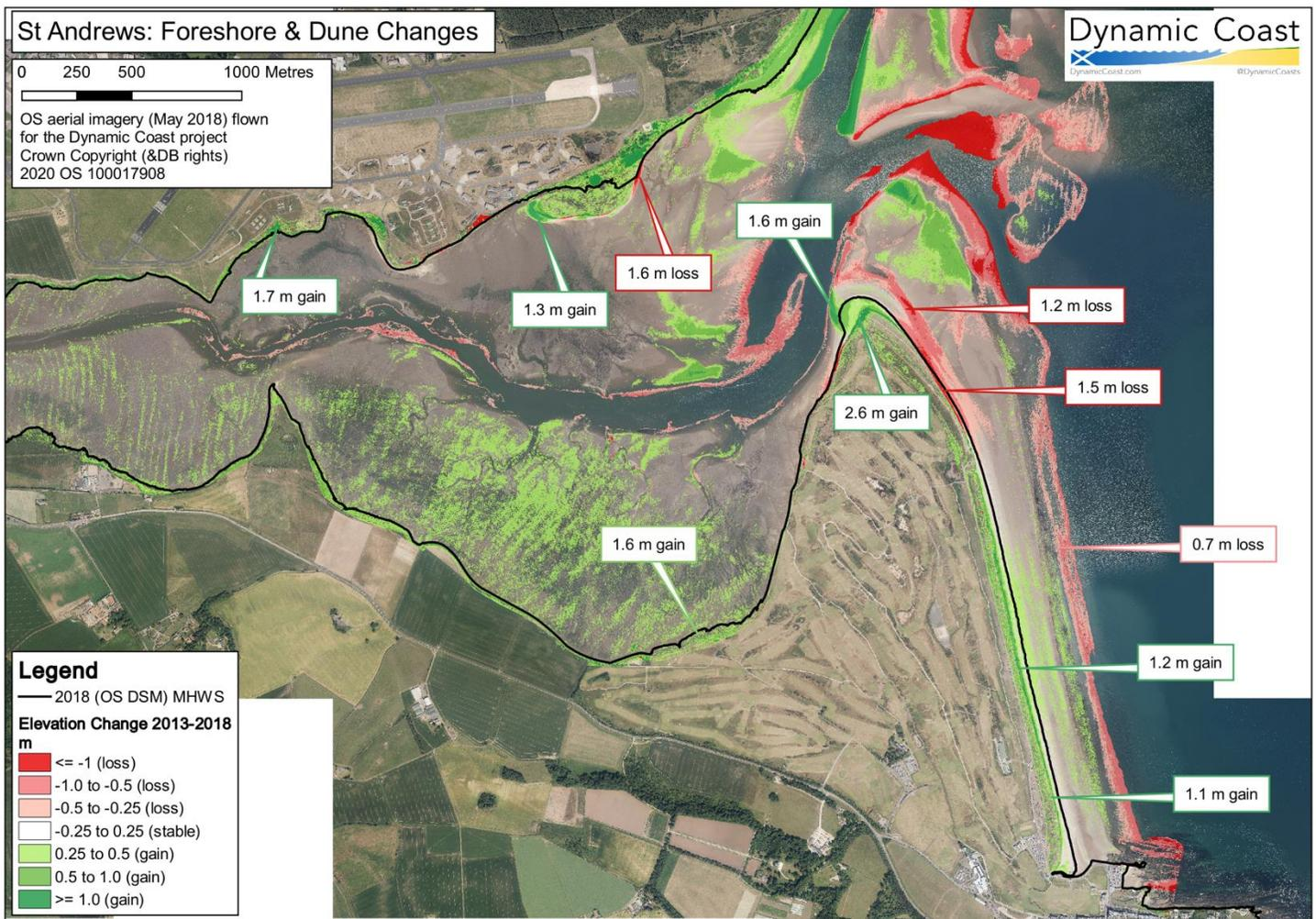
Figure 8 Changes to foreshore elevation - comparison of the difference in beach elevation from 2013 (Scottish Government Phase 2 Lidar) to 2018 (OS DSM from aerial imagery).
