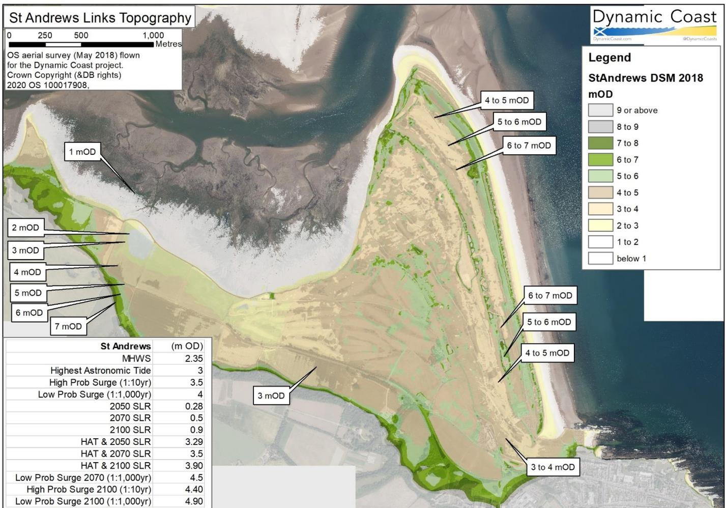
Figure 4 Topography, Bathymetry and key flood levels (mOD) at St Andrews Links.
