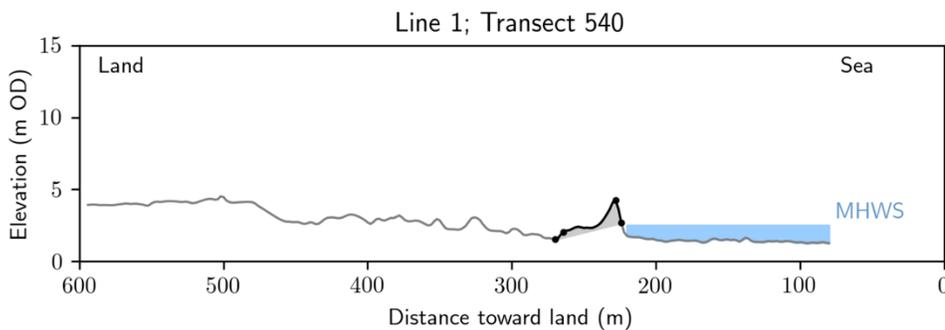
Figure 22 Exempler transect through the Eden Estuary shore showing the narrow embankment protecting low-lying land at great risk from flooding.
