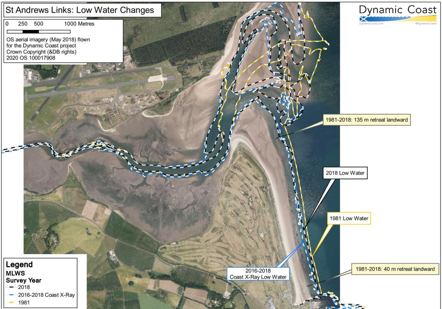
Figure 6 Change to the lower beach – comparison of various MLWS surveys (1882, 1988 & 2018) and Low water (80% water occurrence) from Coast X-Ray.
