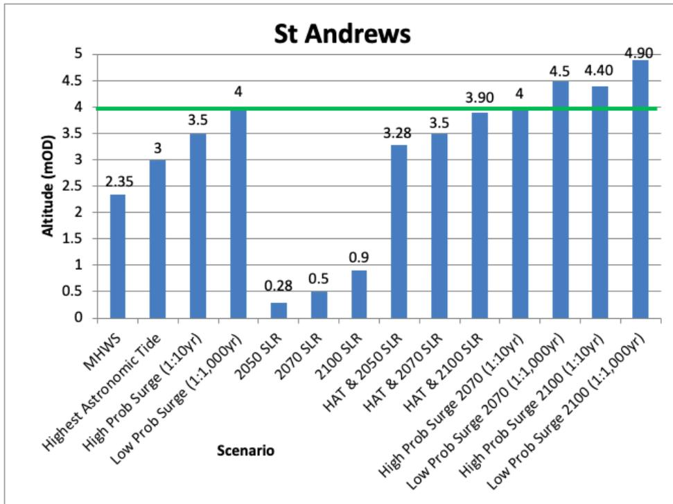
Figure 19 Summary of present and future key tide and flood levels at St Andrews. There are substantial areas of the dune links interior below 4 mOD (annotated with green line) although the dune crest and embankments are higher.
