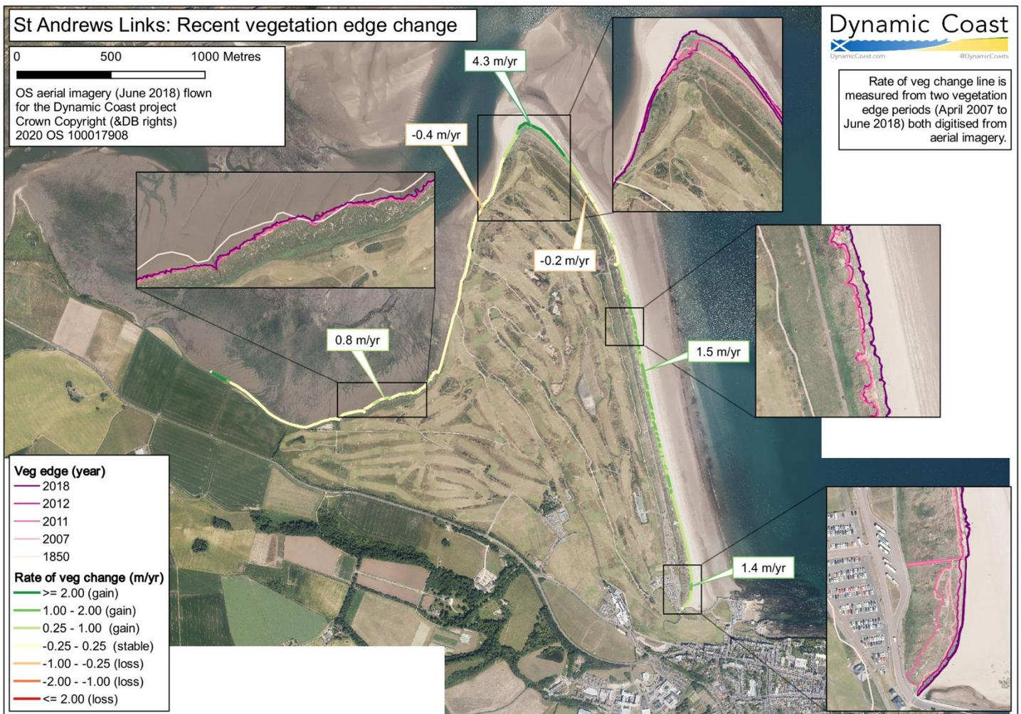
Figure 9 Vegetation edge change maps of St Andrews Links showing observed edges from 1850, 2007, 2011, 2012, and 2018 and the rate of change of distance between 2007 and 2018. Dune infilling accounts for some of this change.
