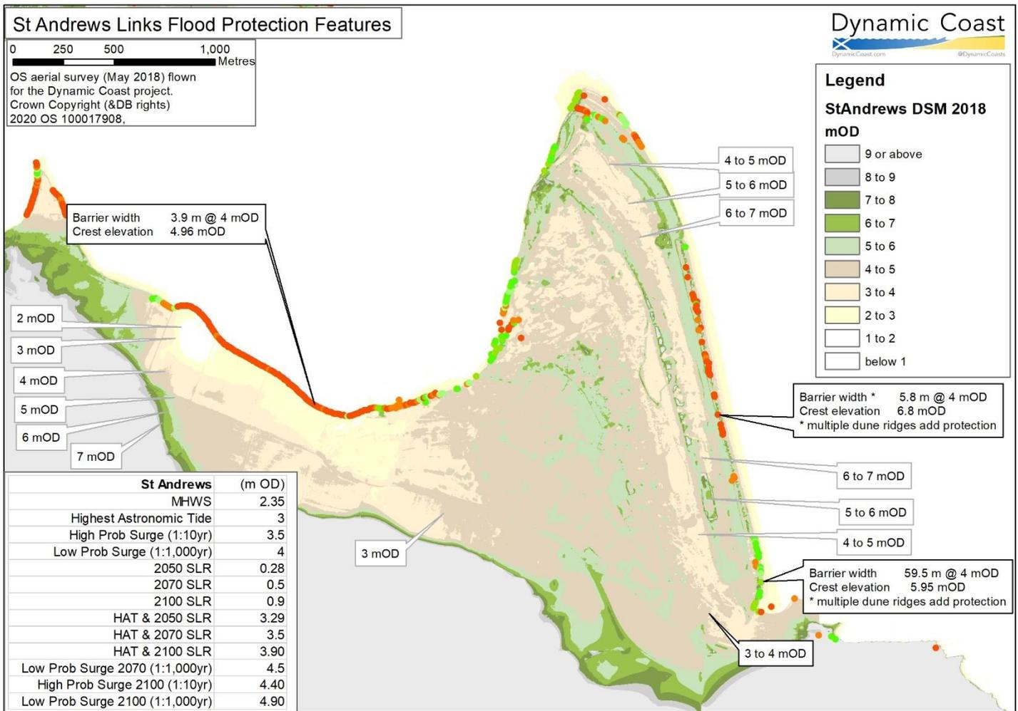
Figure 5 Altitudes of flood protection features at St Andrews Links, showing the extent of the dune cordon (or barrier) (shown by 4 mOD contour). Colour dots identify transects within narrow sections of the dunes or embankments (green dots wide, red dots narrow).
