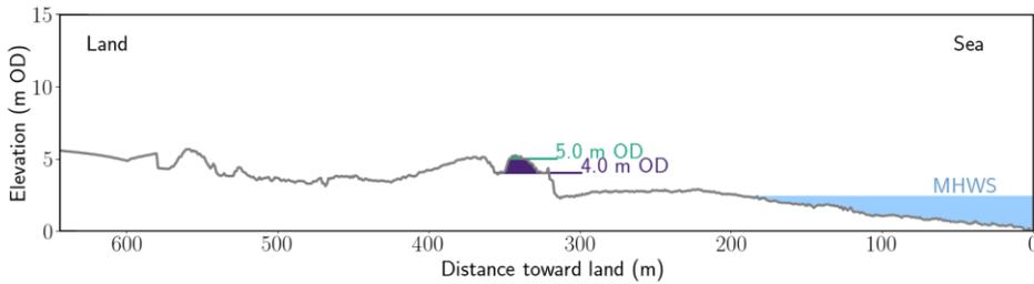
Figure 21 Exempler transect through the Swilcan Burn area showing the narrow ridge (with the road, highlighted). The lower interior is connected to the sea via the Swilcan burn. The 18<sup>th</sup> green of the Old Course lies at 400–500 m on this transect.
