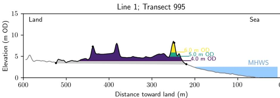
Figure 20 Exemplar transect through the West Sands dune cordon of multiple dune ridges, each providing a flood protection function. These ridges are shown as green areas in Figure 5. Key attributes are annotated along with the volume above certain elevations (a proxy for resilience).
