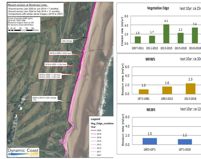
Figure 9 Detailed vegetation edge change following Storm Brendan (ca. 12<sup>th</sup> to 14<sup>th</sup> January 2020) compared with recent ground survey and aerial photography analysis.
