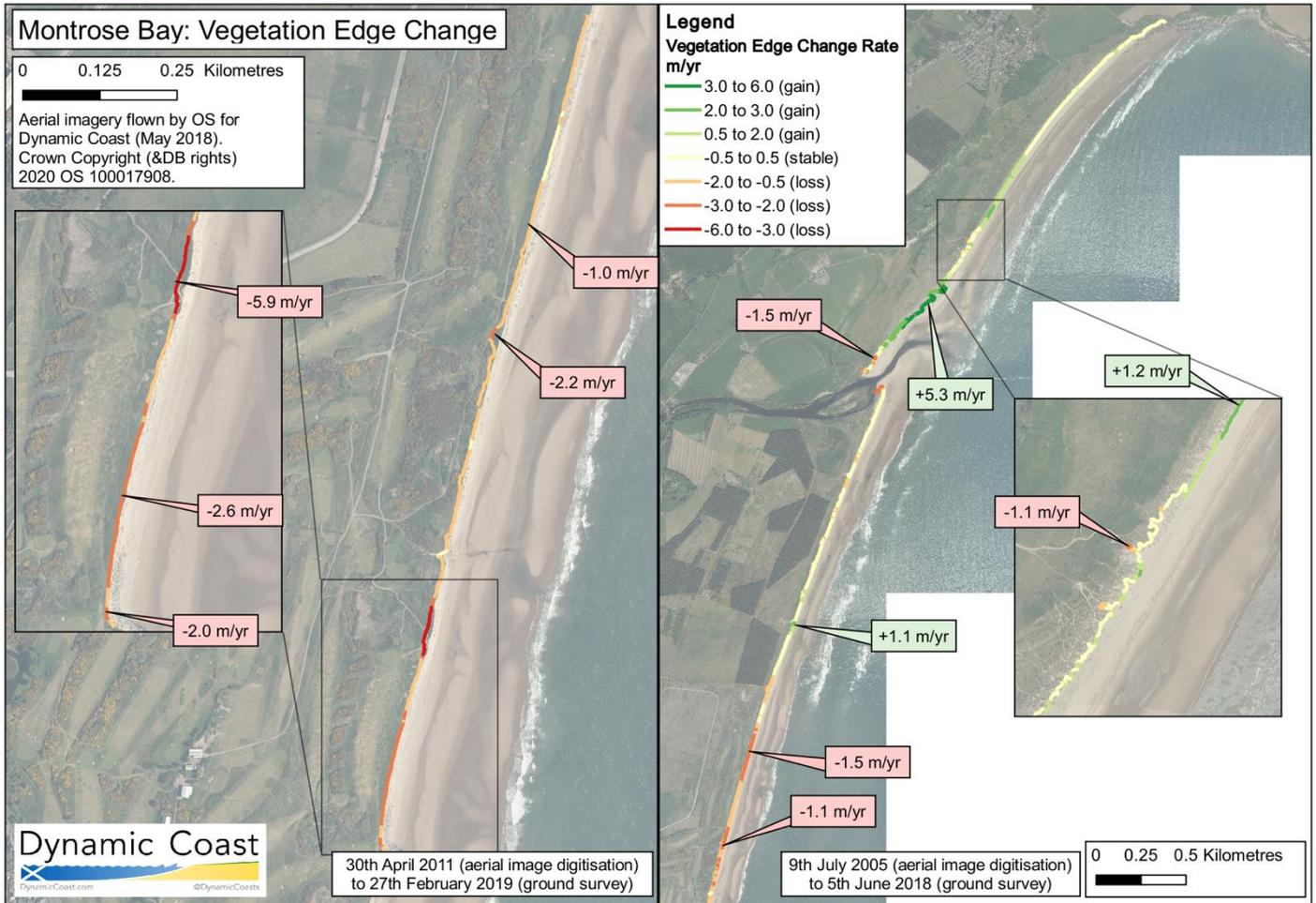
Figure 8 Vegetation edge change at Montrose Bay (2011 to 2019 and 2005 to 2018). Note the -5.9 m retreat which reflects the retreat of the vegetation edge following the removal of the rock armour at this location.
