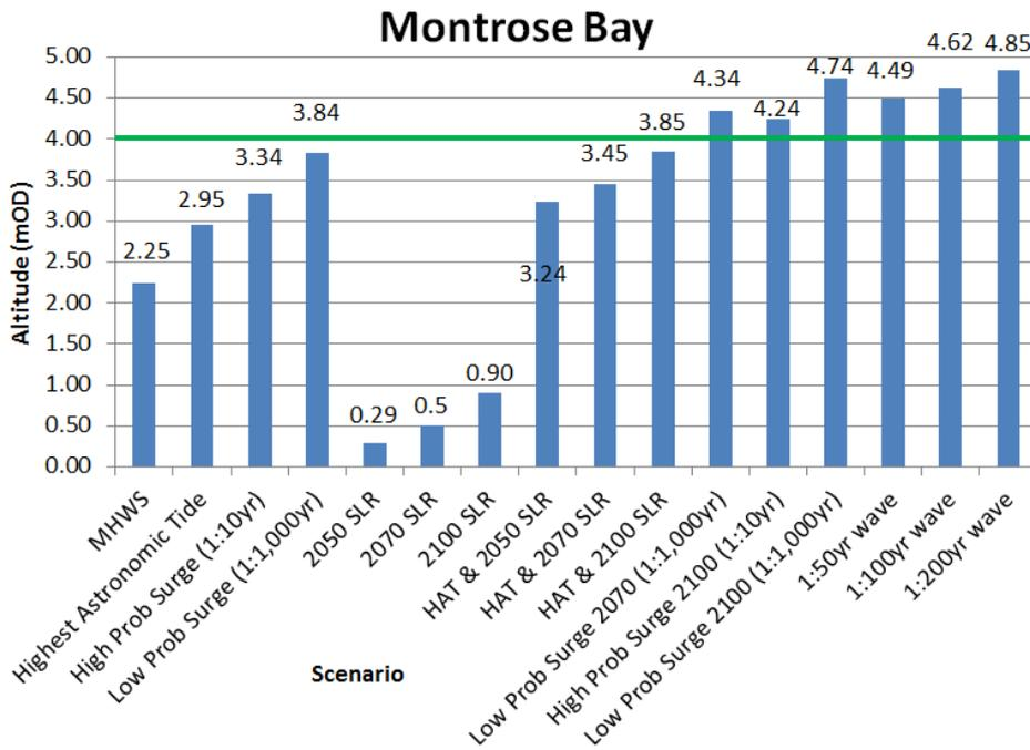
Figure 20 Summary of future key tide and flood levels at Montrose Bay. There are substantial areas of the dune interior across the bay below 4 mOD (annotated with green line)
