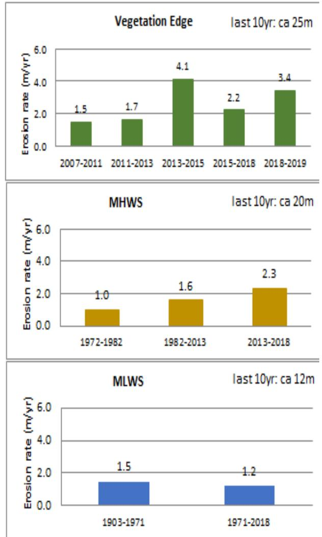
Figure 10 Comparison of rates of change – Vegetation Edge, Mean High Water Springs and Mean Low Water Springs.
