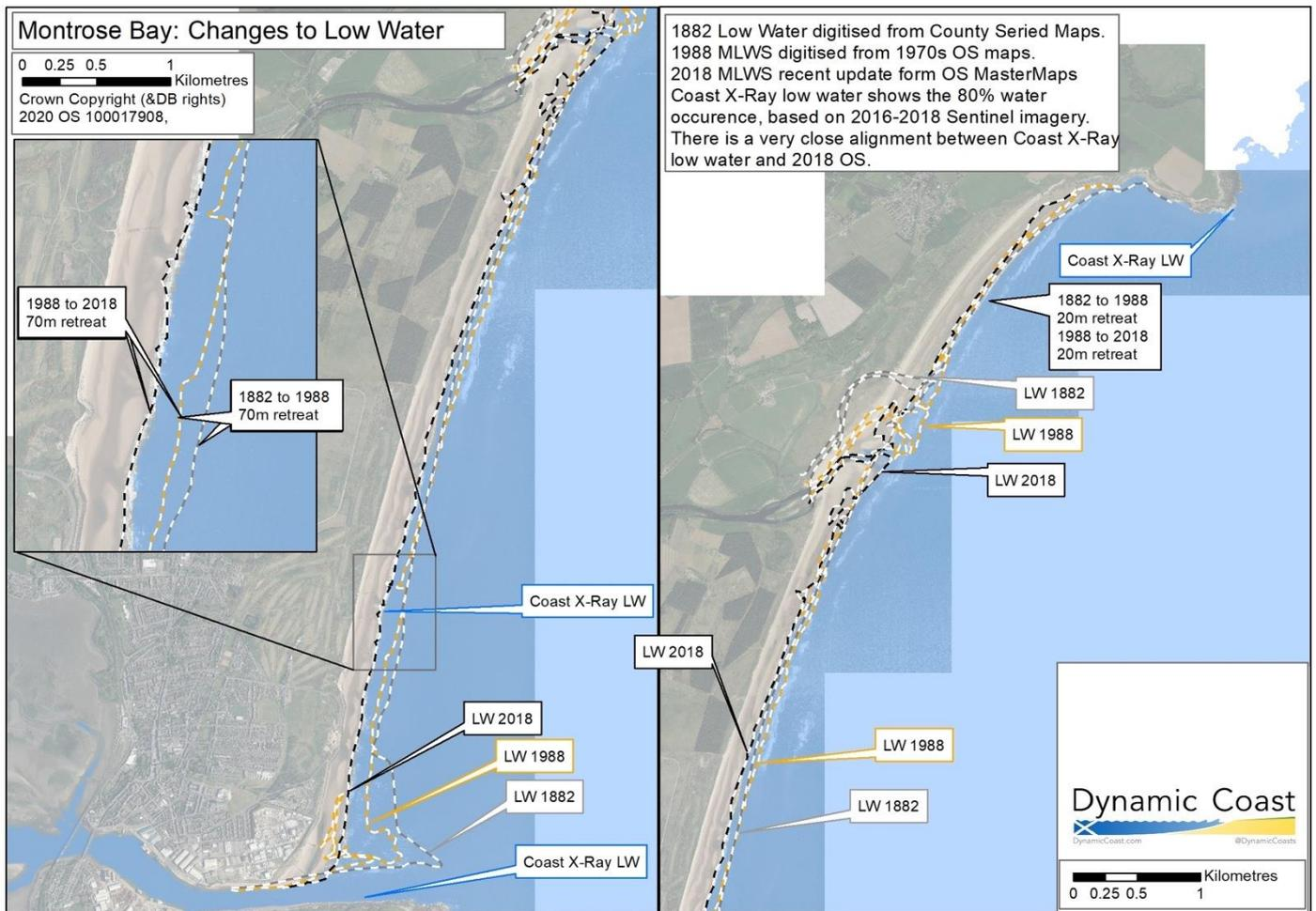
Figure 5 Change to the lower beach – comparison of various MLWS surveys (1882, 1988 & 2018) and Low water (80% water occurrence) from Coast X-ray
