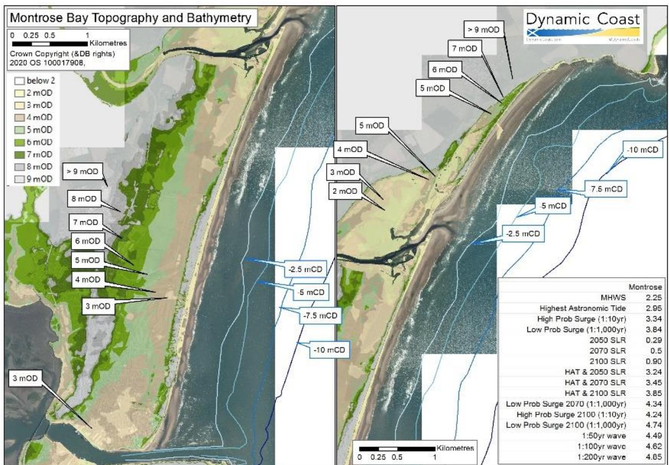
Figure 3 Topography, Bathymetry and key flood levels (mOD) within Montrose Bay.
