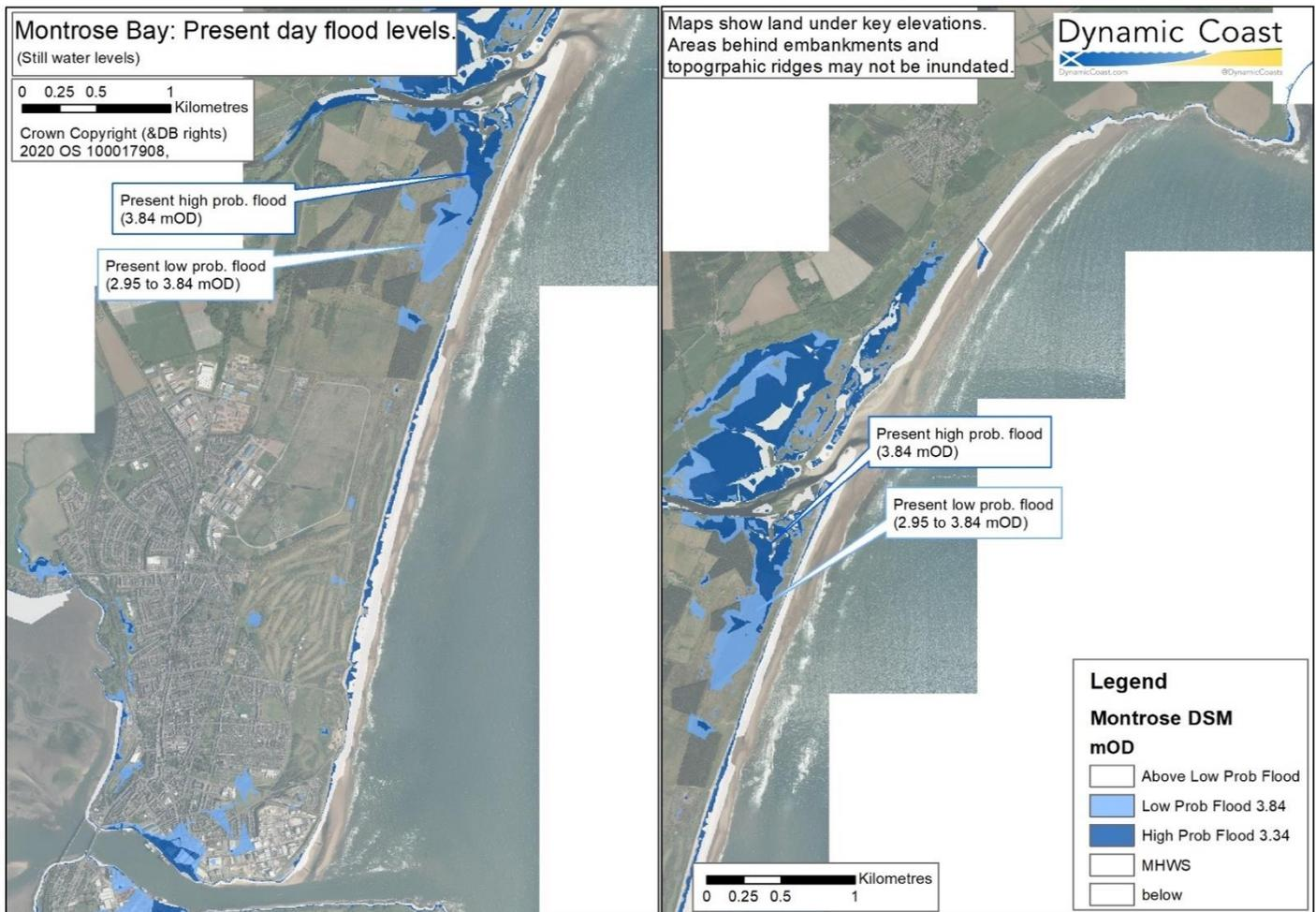
Figure 17 Summary of present day high probability (1:10 yr 3.34 mOD) and low probability (1:1,000 yr 3.84 mOD) flood levels at Montrose Bay.
