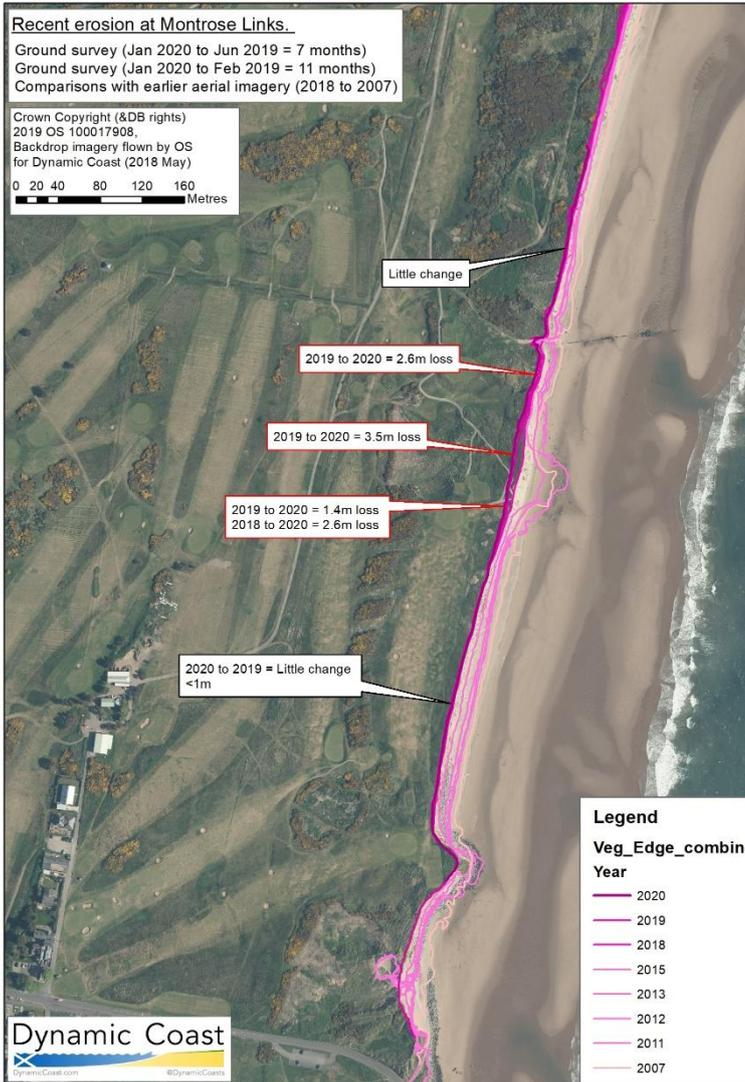
Figure 9 Detailed vegetation edge change following Storm Brendan (ca. 12<sup>th</sup> to 14<sup>th</sup> January 2020) compared with recent ground survey and aerial photography analysis.
