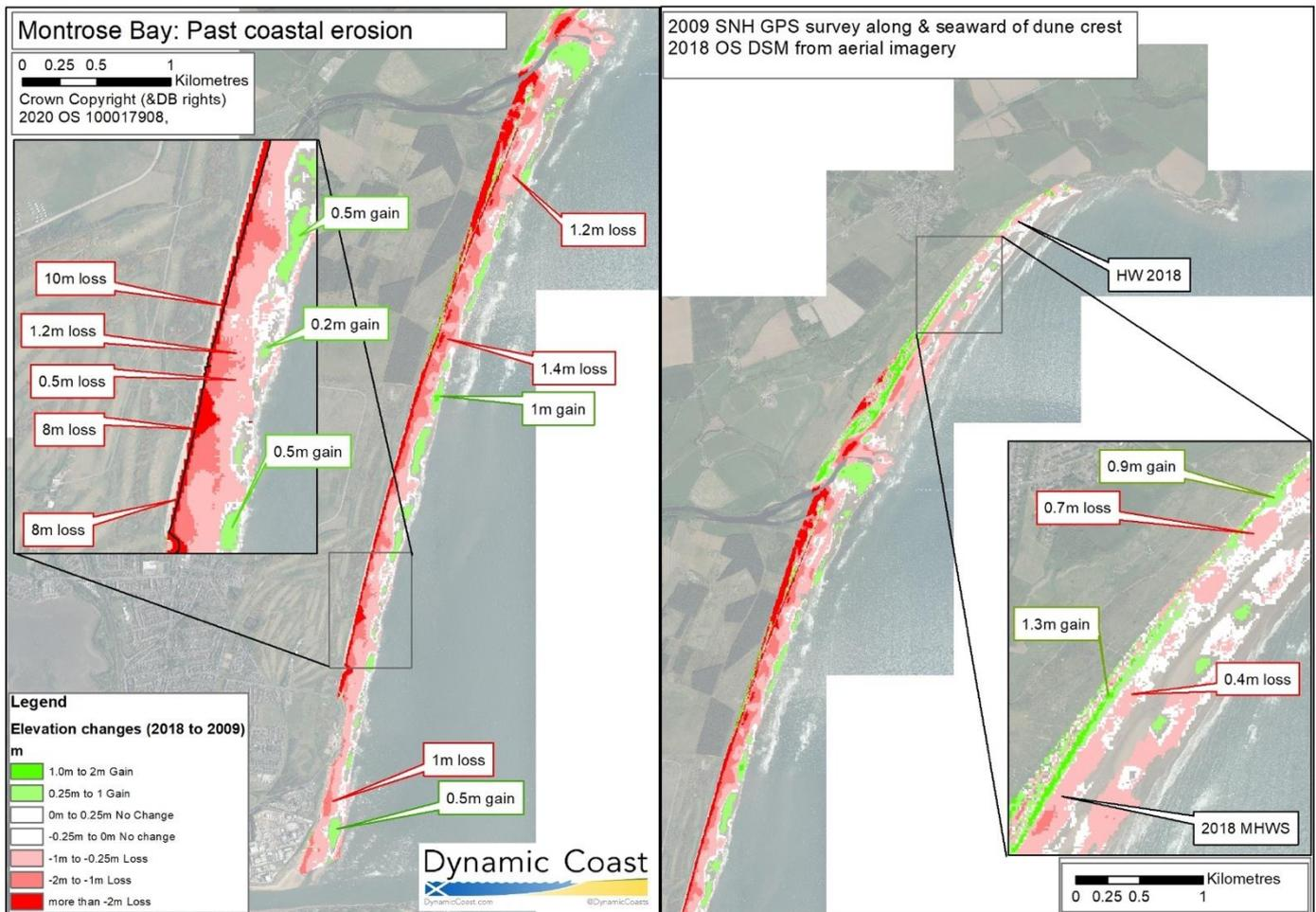
Figure 7 Changes in foreshore elevation from 2009 (SNH GPS survey seaward of dune crest) to 2018 (OS DSM from aerial imagery).
