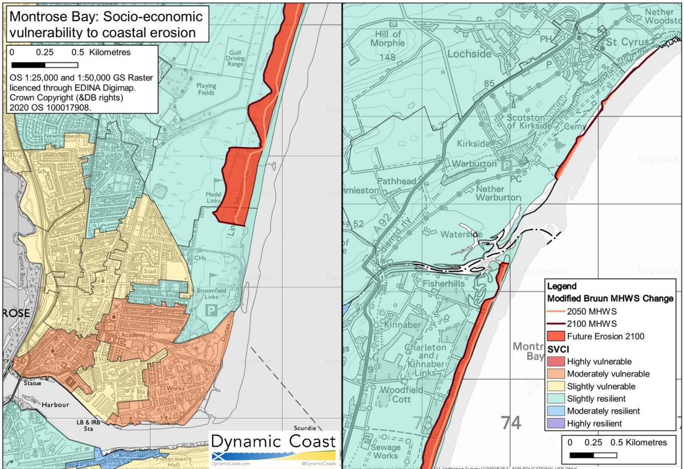
Figure 16 SVCI classifications per data zone with anticipated coastal change using the Modified Bruun Rule
