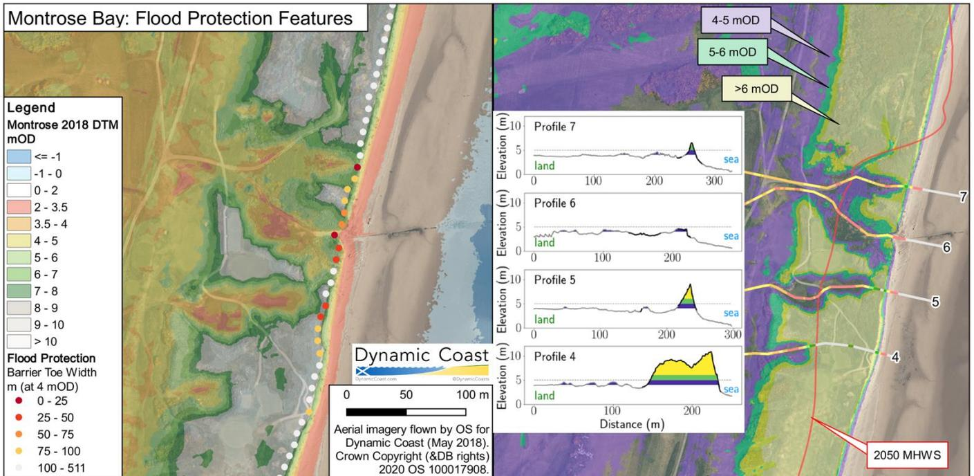
Figure 21 Identification of flood corridors within the southern section of dunes.
