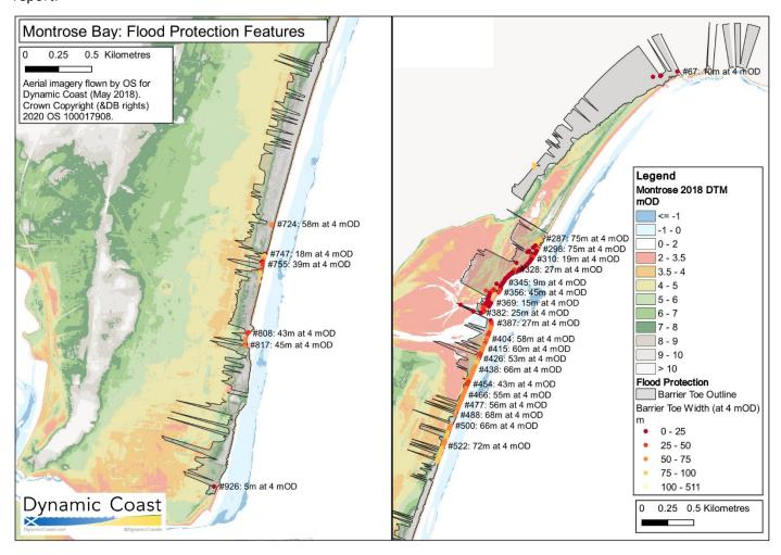
Figure 4 Flood protection features at Montrose, showing the extent of the barrier toe (grey box) and the front points of barriers symbolised by the width of each barrier at 4 mOD. Barrier toe width of narrowest barriers is annotated alongside transect number.
