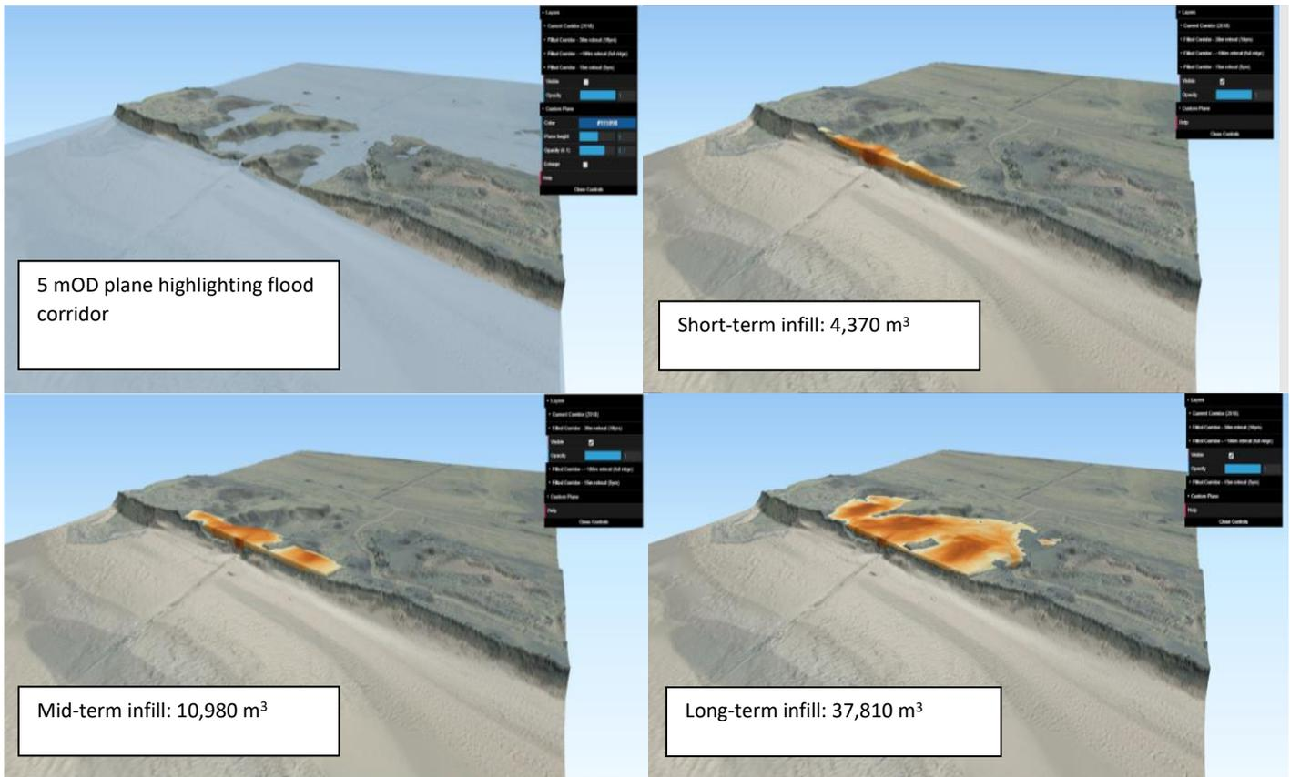
Figure 22 Sediment infill and dune reprofiling options within the southern section of Montrose dunes (NOTE: short, mid and long term options could be enacted immediately).
