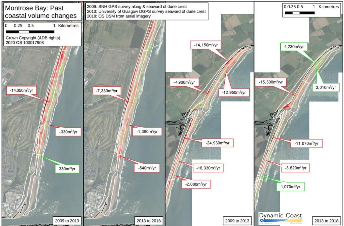
Figure 11 Comparison of rates of volume change across each geomorphic section outlined in white, from 2009 to 2013 and 2013 to 2018
