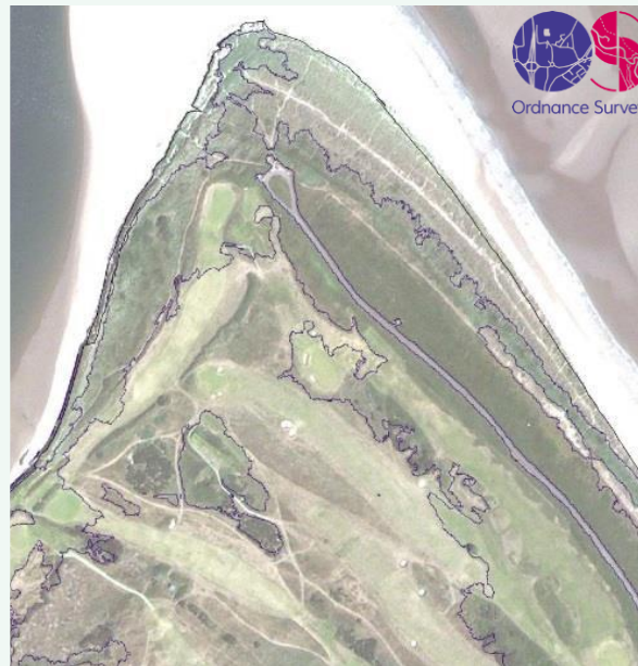
Automatic veg edge detection on satellite & aerial imagery
