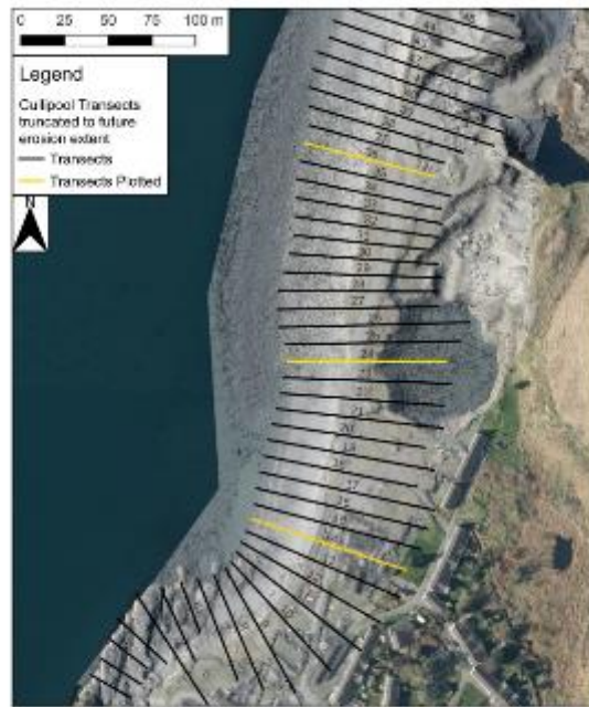
Figure 9. Transects used for shoreline change analysis. Transects are numbered sequentially from south to north. Transects 14, 24 and 36 highlighted were selected to visualise cross-shore topographic profiles as shown in Figure 10.
