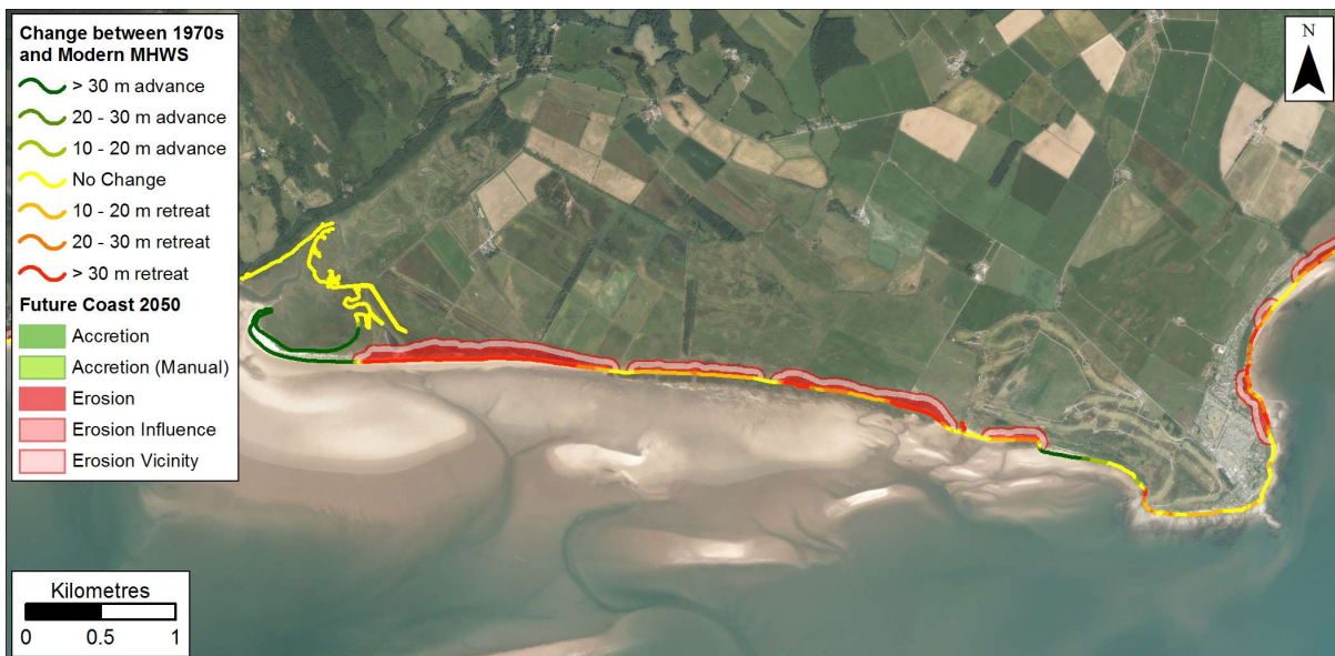
Figure 7.12: Possible future coastline position in 2050 based on rates between 1970 and Modern MHWs data from Mersehead Sands to Southerness. Getmapping are our current providers of Scotland-wide digital aerial imagery© Getmapping plc.
