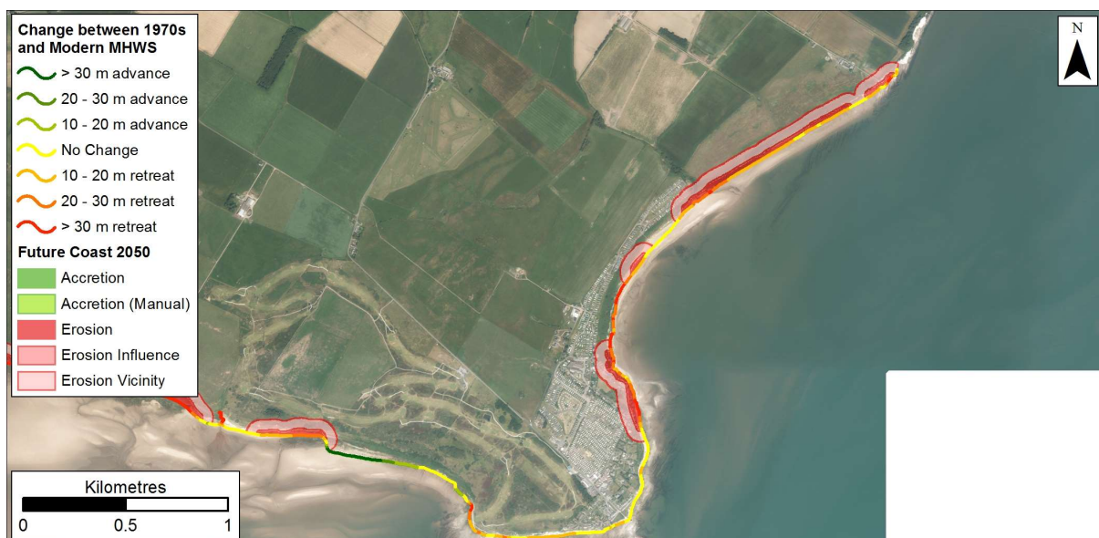
Figure 7.14: Possible future coastline position in 2050 based on rates between 1970 and Modern MHWS data at Southernness. Getmapping are our current providers of Scotland-wide digital aerial imagery © Getmapping plc.
