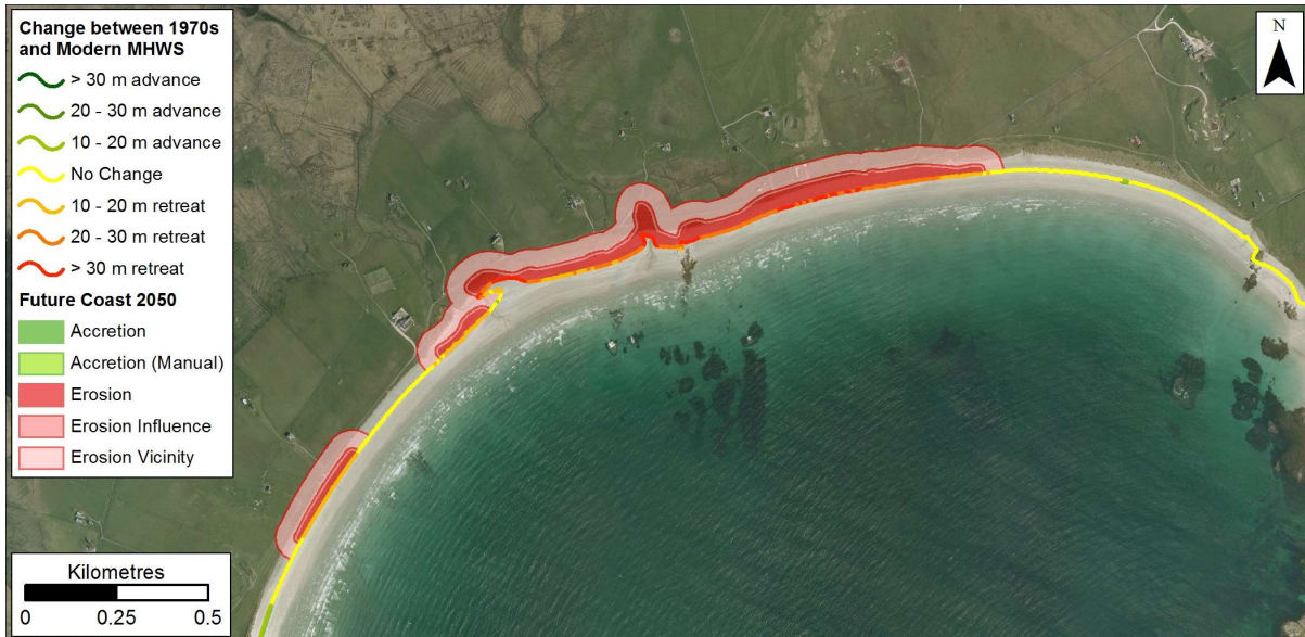
Figure 5.36: Possible future coastline position in 2050 based on rates between 1970 and Modern MHWS data at Traigh Mhor. Getmapping are our current providers of Scotland-wide digital aerial imagery © Getmapping plc.
