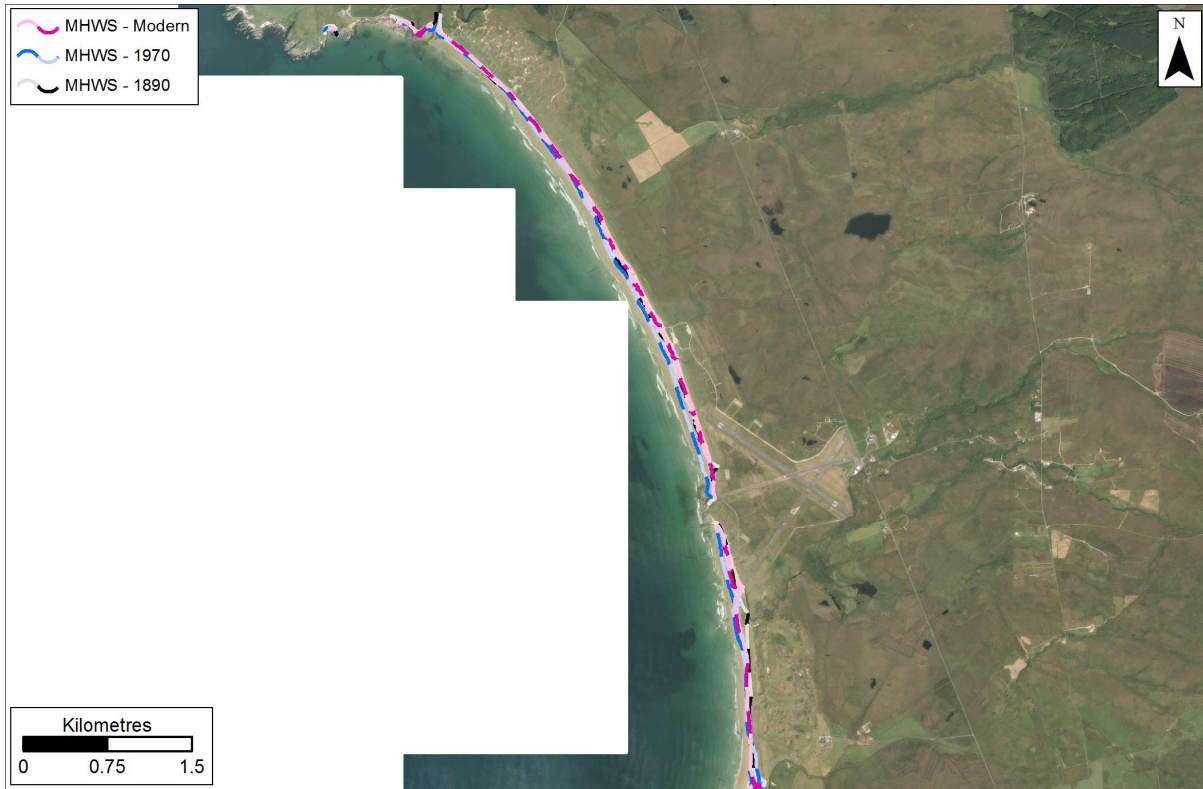
Figure 5.25: MHWS position in 1890, 1970s, and Modern datasets at Laggan Bay. Getmapping are our current providers of Scotland-wide digital aerial imagery© Getmapping plc.
