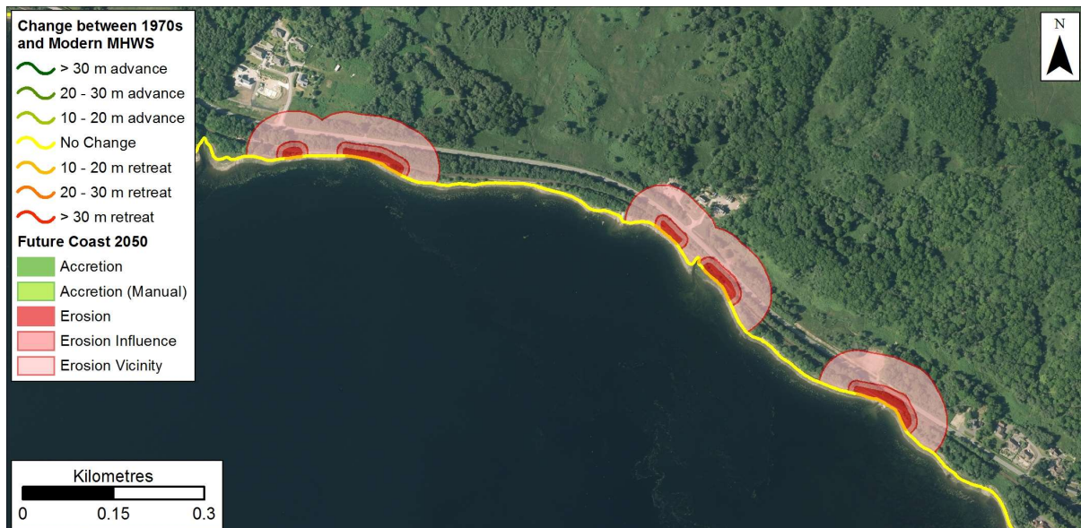
Figure 5.18: Possible future coastline position in 2050 based on rates between 1970 and Modern MHWS data at Corpach. Getmapping are our current providers of Scotland-wide digital aerial imagery© Getmapping plc.
