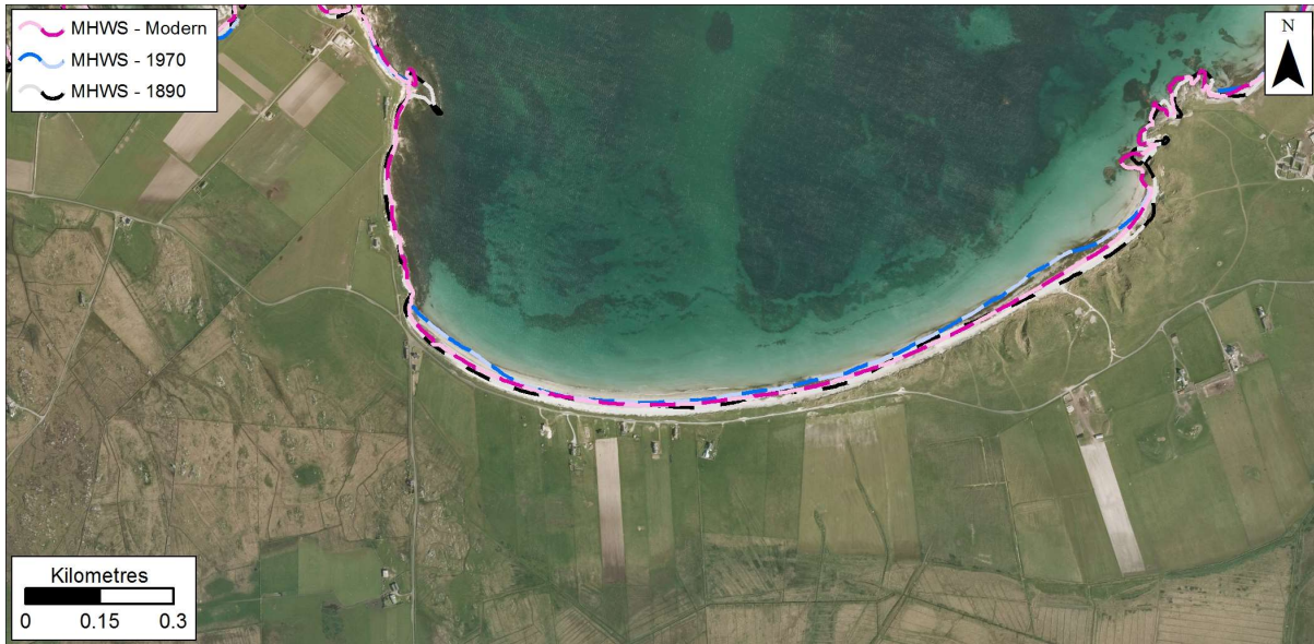
Figure 5.37: MHWS position in 1890, 1970s, and Modern datasets at Balephetrish Bay. Getmapping are our current providers of Scotland-wide digital aerial imagery© Getmapping plc.
