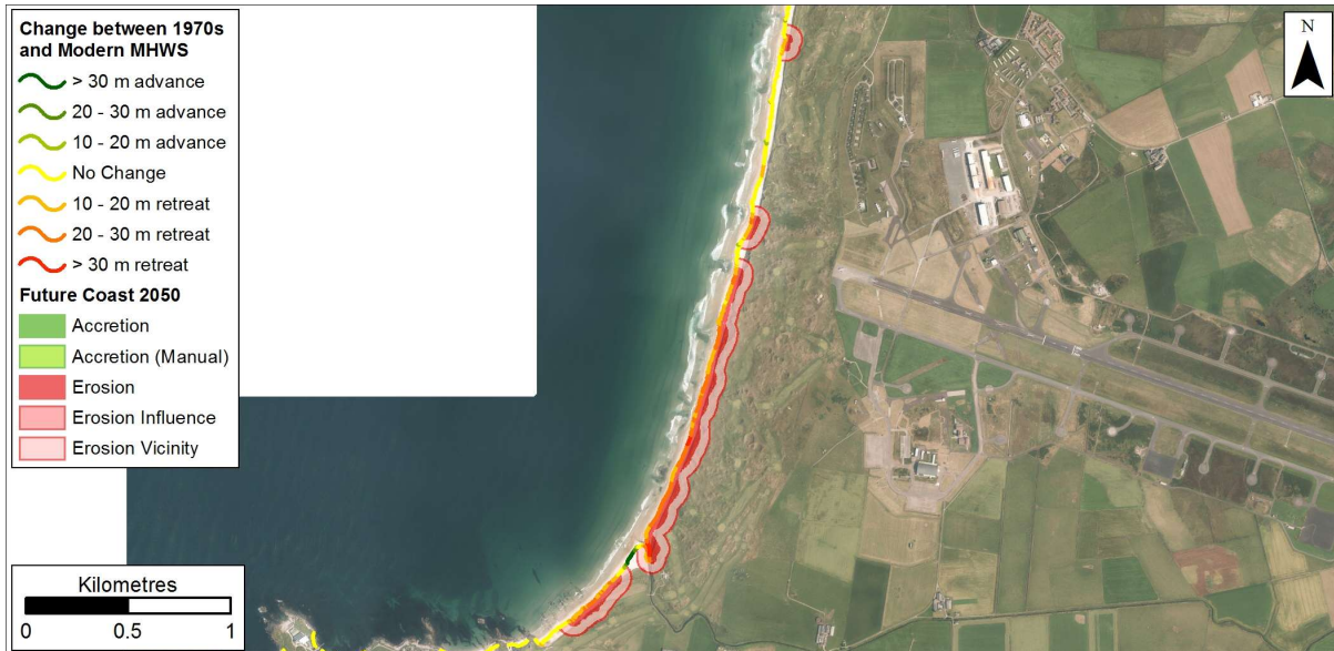
Figure 5.24: Possible future coastline position in 2050 based on rates between 1970 and Modern MHWS data at Machrihanish. Getmapping are our current providers of Scotland-wide digital aerial imagery© Getmapping plc.
