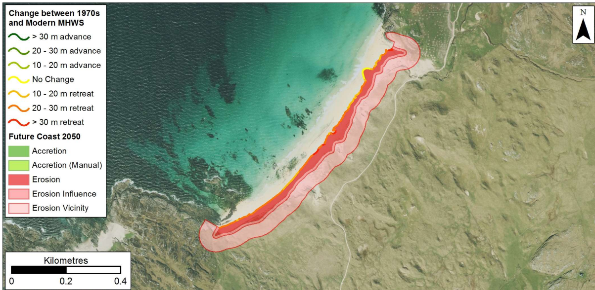
Figure 5.31: Possible future coastline position in 2050 based on rates between 1970 and Modern MHWS data at Hough. Getmapping are our current providers of Scotland-wide digital aerial imagery © Getmapping plc.
