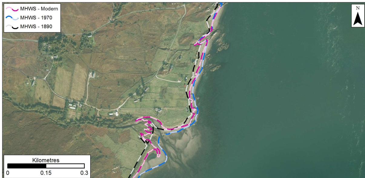
Figure 5.15: MHW position in 1890, 1970s, and Modern datasets at Kylerhea. Getmapping are our current providers of Scotland-wide digital aerial imagery© Getmapping plc.
