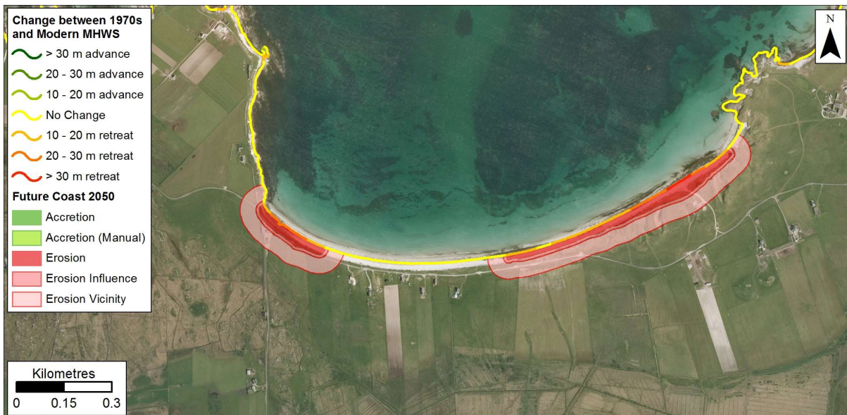
Figure 5.38: Possible future coastline position in 2050 based on rates between 1970 and Modern MHWS data at Balephetrish Bay. Getmapping are our current providers of Scotland-wide digital aerial imagery© Getmapping plc.
