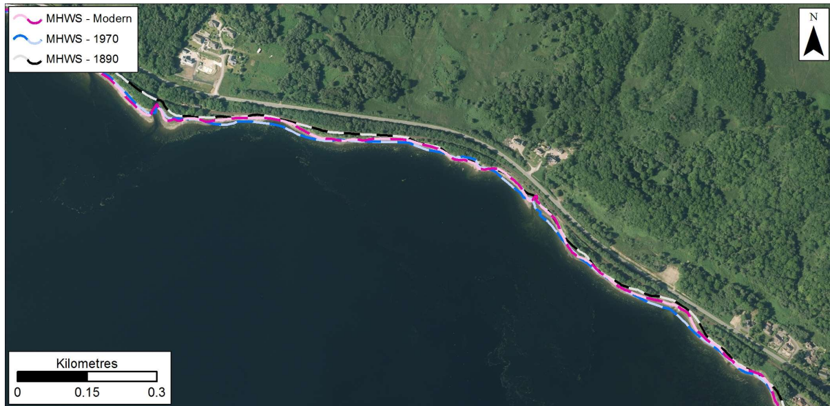
Figure 5.17: MHWS position in 1890, 1970s, and Modern datasets at Corpach. Getmapping are our current providers of Scotland-wide digital aerial imagery© Getmapping plc.
