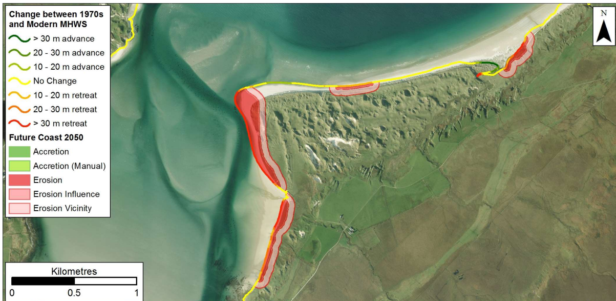
Figure 5.28: Possible future coastline position in 2050 based on rates between 1970 and Modern MHWs data at Killinallan Point. Getmapping are our current providers of Scotland-wide digital aerial imagery© Getmapping plc.
