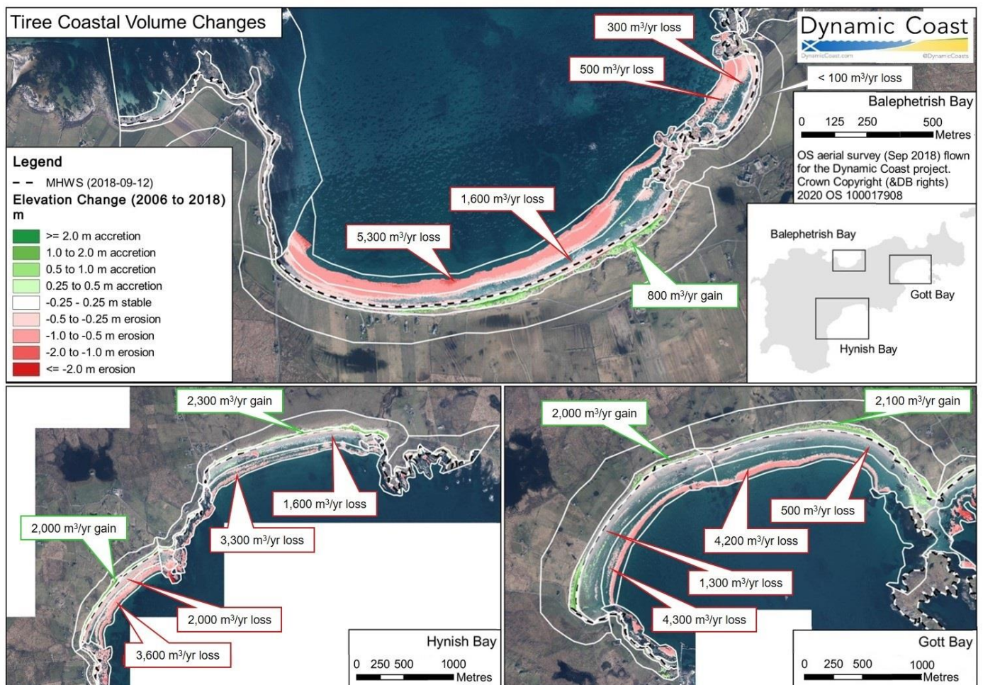
Figure 10 Comparison of rates of volume change across each geomorphic section outlined in white, from 2006 (SNH Lidar) to 2018 (OS aerial DSM)
