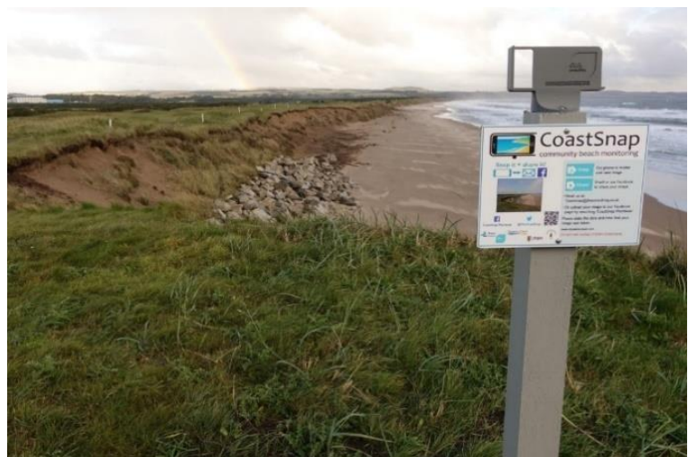
Figure 3 Montrose Links CoastSnap post which allows members of the public to take and share fixed point photography. Such citizen science complements ground and aerial analysis. © J.Adams / D.Pender {TBC}.
