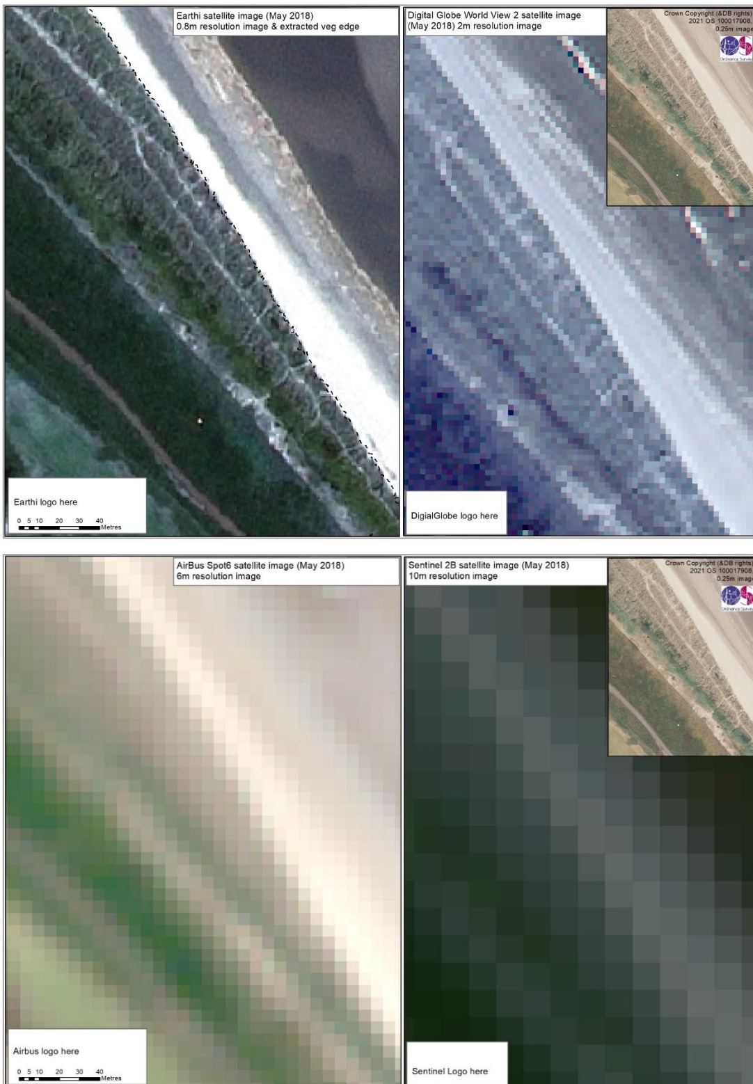
Figure 9 comparison of remote sensed data and vegetation edge extracted from Earth-I image (top left) 0.8m pixel size (pan sharpened) compared with (nominal multispectral resolution) 2m pixel (top right from Digital Globe), 6m (bottom left from Airbus Spot6) and 10m pixel (bottom right from Sentinel 2b) inset shows OS aerial imagery (0.25m pixel size).
