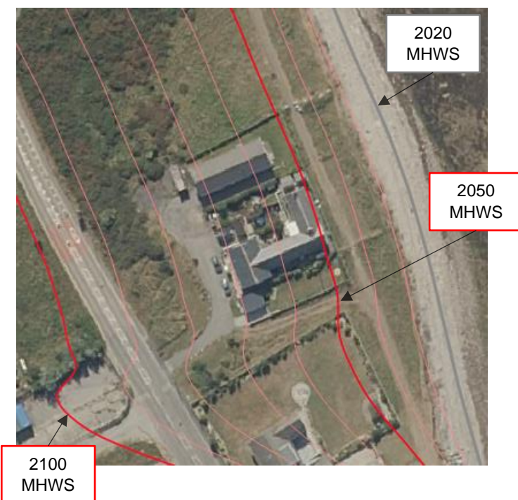
Figure 1 Exemplar location with buildings, road and associated infrastructure at risk from anticipated erosion. Grey line represents 2020 MHWS, pink lines are decadal anticipated MHWS positions from 2030 inland (right to left) with 2050 and 2100 marked in bold red. Anticipated retreat is under a high emission scenario and a 'do nothing' coastal management scenario. Indicative Results.
